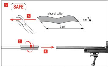
Put the safety on "safe". Prepare a thin rod with a length of approx. 60 cm. Attach a piece of cotton fabric to its end and clean the barrel with some silicone oil.
